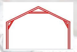
The Structural steel building frame consists of columns and rafters. The column and rafter are typically tapered being narrow at the foundation and peak and wider at the rafter/column connection.
