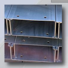
cold formed components are engineered specifically for the building location. The main frame steel will vary from 4" to 24" in depth and 2 ½ to 5" wide, the gauge varies from 16ga to 10ga.
